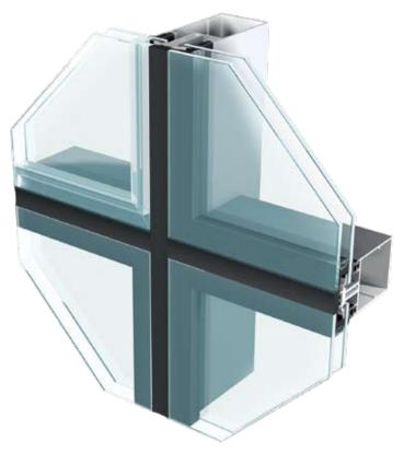
Elegance 52 SX is a structurally clamped aluminium curtain wall system where the glass is retained directly towards the standard structure of Elegance 52 ST with the use of concealed pressure plates. The retained intercalary profile between the double glazed panes provides the area to insert the pressure plates which are directly screwed in the central groove of the mullions and transoms.
