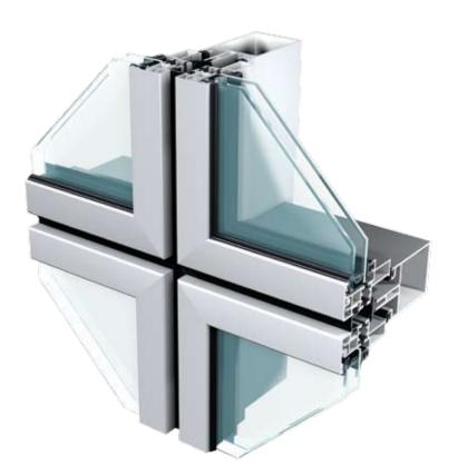
Elegance 52 GF is a curtain wall system based on the structure of the Elegance 52 SG using a glazing bead instead of structurally glazing the glass to the panel. The design team developed this solution to offer a version where the glass is held in position with aluminium as in a picture frame. This approach allows each panel to be independent but still be integrated in the full curtain wall.
