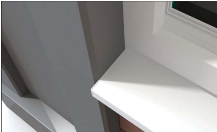
150mm PVC cill against large column. Endcaps are required as cill will overhang the column claddings
