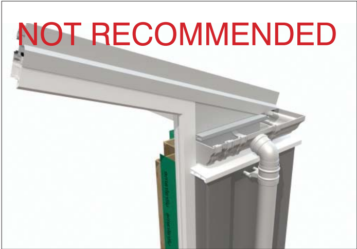
SHORT RETURN WITH CILL. If unable to return back to house wall use inline outlet for 67° obtuse round, positioned centrally on column.
