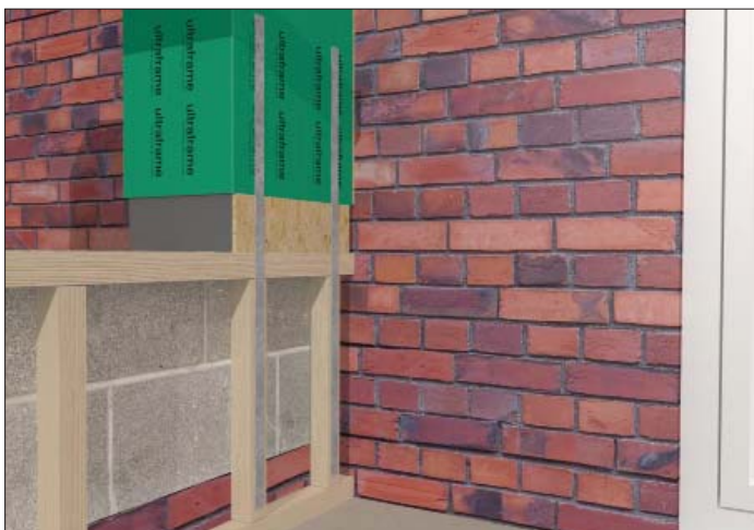
STRAPS MUST LINE UP WITH STUDWORK
