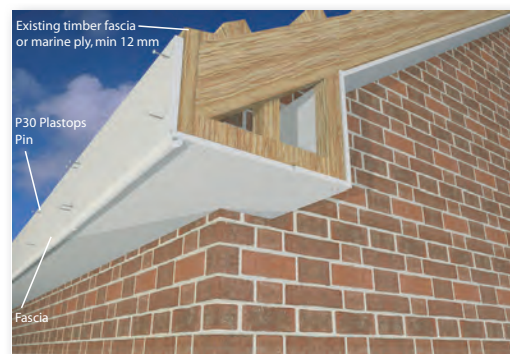
Fig. 17. Standard over-fascia installation.
